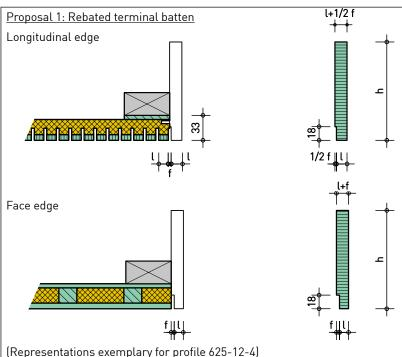
In this example, the terminal batten is laterally butt-joined. It is fastened e.g. using nails or small clamps
