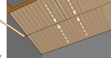
If special NF type elements are being used, this cut <u>must</u> take place in any case, because otherwise, the gap width at the lateral element joint does not exactly correspond to the gap width in the element surface.
