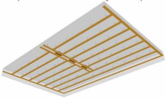
Installation substructure directly to the building structure,
